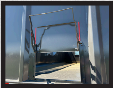
MANUAL LIFT GRAIN DOOR
